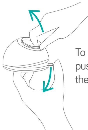
To disassemble push down on the lip.
