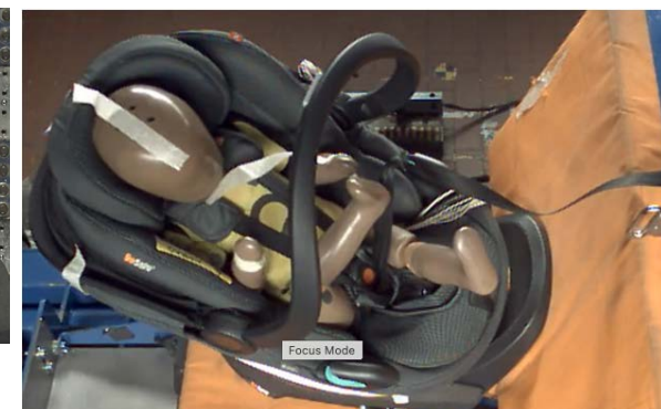
Out of position test
