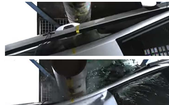
Euro NCAP side pole test example
